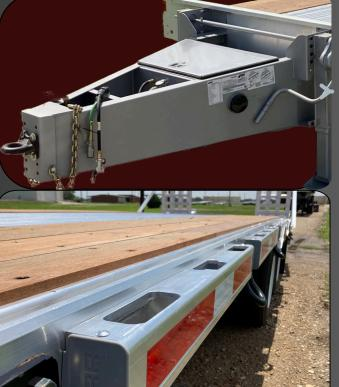
Doonan replaced the steel gooseneck used on its Chaparral II drop deck trailers with a galvanized steel A-frame pintle hitch (tongue /drawbar) to providing unmatched corrosion protection.
