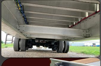
The Chaparral II Tag trailer series uses the same aluminum main beam, crossmember, and side rail extrusions that have been used in the Chaparral II Class 8 drop deck trailers since 2013.
