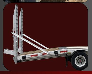
Doonan utilizes custom aluminum ramps to achieve an 8-degree angle providing for easy equipment loading and unloading. The spring assisted light weight ramp is extremely easy to Lift, Lower and Slide side to side minimizing any potential injury to operator.
